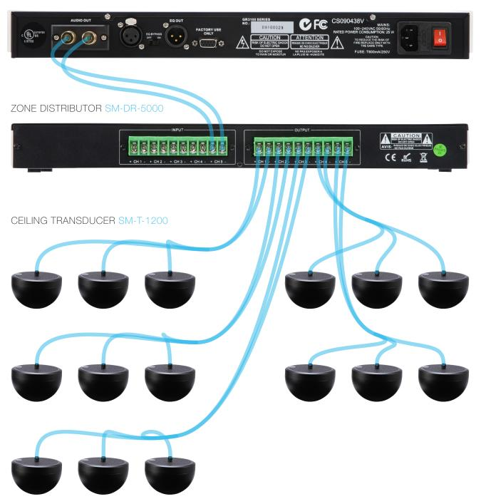
NOTES > The SM-DR-5000 is capable of servicing up to 100 transducers for each generator. > Diagram not to scale.
