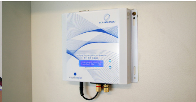
Soundmask's shelf generator SM-GS-3200 affixed to wall
