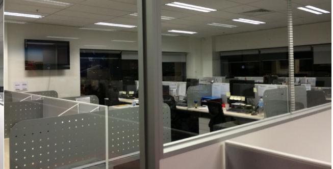
The sales call centre was encased in glass windows, which increased the reverberation and noise levels
